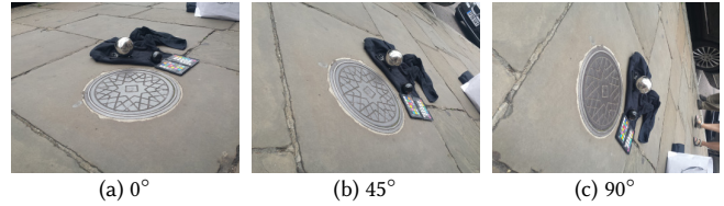
Fig. 9. Polarization measurements with hand-held acquisition with a mobile phone. A static polarizer is mounted in front of the lens and the entire device is rotated in-plane to the desired 0^\circ , 45^\circ , and 90^\circ orientations to acquire the data.
