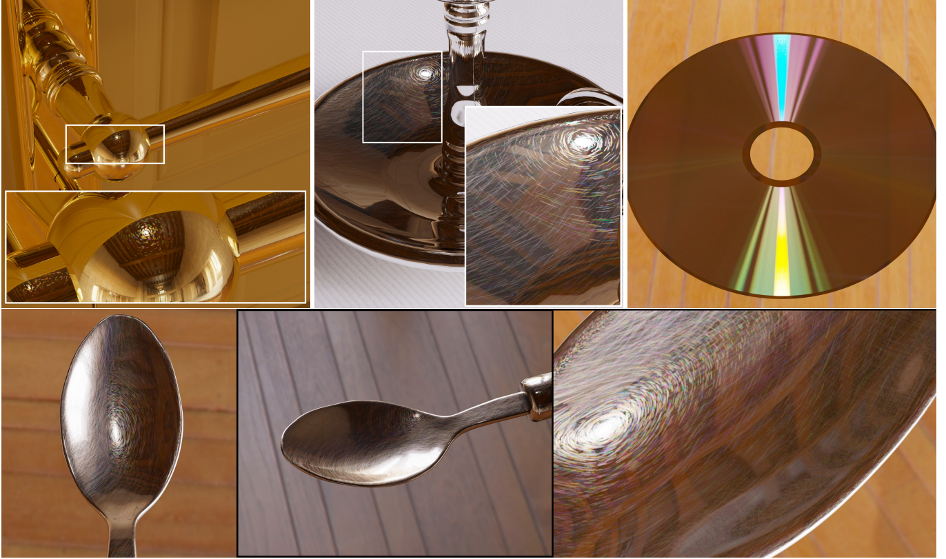
Fig. 6. We demonstrate our reflectance model on four example scenes. Top row from left to right: A golden door handle, a candle holder, both with randomized scratch distributions. A compact disc with circular scratches with constant separation. Bottom row: A spoon from different view points, the scratches are randomized. The top-down view reveals the scratches with iridescent colors that lie on a circle around the specular highlight. In the side-view the specular highlight only subtends a small fraction on the spoon and under incoherent illumination by the surrounding lights the scratches appear mostly white. At close-up again color as well as geometry of the scratches is revealed. We present complementary videos for these scenes in the supplemental material.
