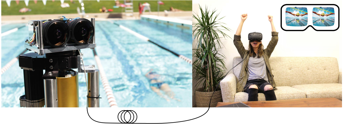
Fig. 1. We present Vortex, an architecture for live-streaming 3D virtual reality video. Vortex uses two fast line sensors combined with wide-angle lenses, spinning at up to 300 rpm, to directly capture stereoscopic 360° virtual reality video in the widely-used omni-directional stereo (ODS) format. In contrast to existing VR capture systems, no expensive post-processing or complex calibration are required, enabling live streaming of high quality 3D VR content. We capture a variety of example videos showing indoor and outdoor scenes and analyze system design tradeoffs in detail.
