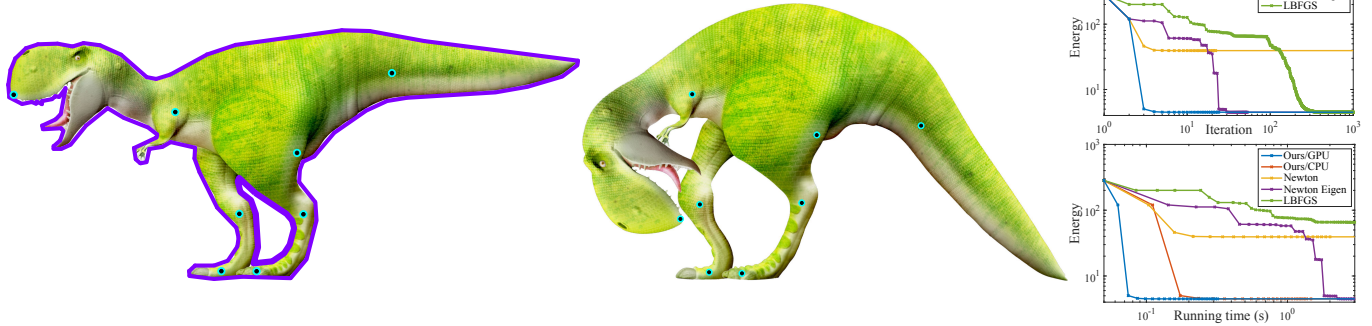
Fig. 1. Locally injective isometric deformation of Rex, a doubly-connected planar domain (left). Note the hole between the legs. Our harmonic subspace has 392 DOF. Our solver converges after 6 iterations to the result depicted, which is computed in 0.072s when implemented on the GPU, and 0.375s on the CPU. We compare against an unmodified Newton solver which halts prematurely after 9 iterations at a high energy configuration due to a non-positive definite Hessian. The Newton-Eigen solver performs a full eigen-factorization Hessian modification at each iteration. It converges after 32 iterations and takes 2.467s which is \times 34 times slower than our GPU solver. The L-BFGS solver performs 1,818 iterations and is not competitive in terms of runtime.
