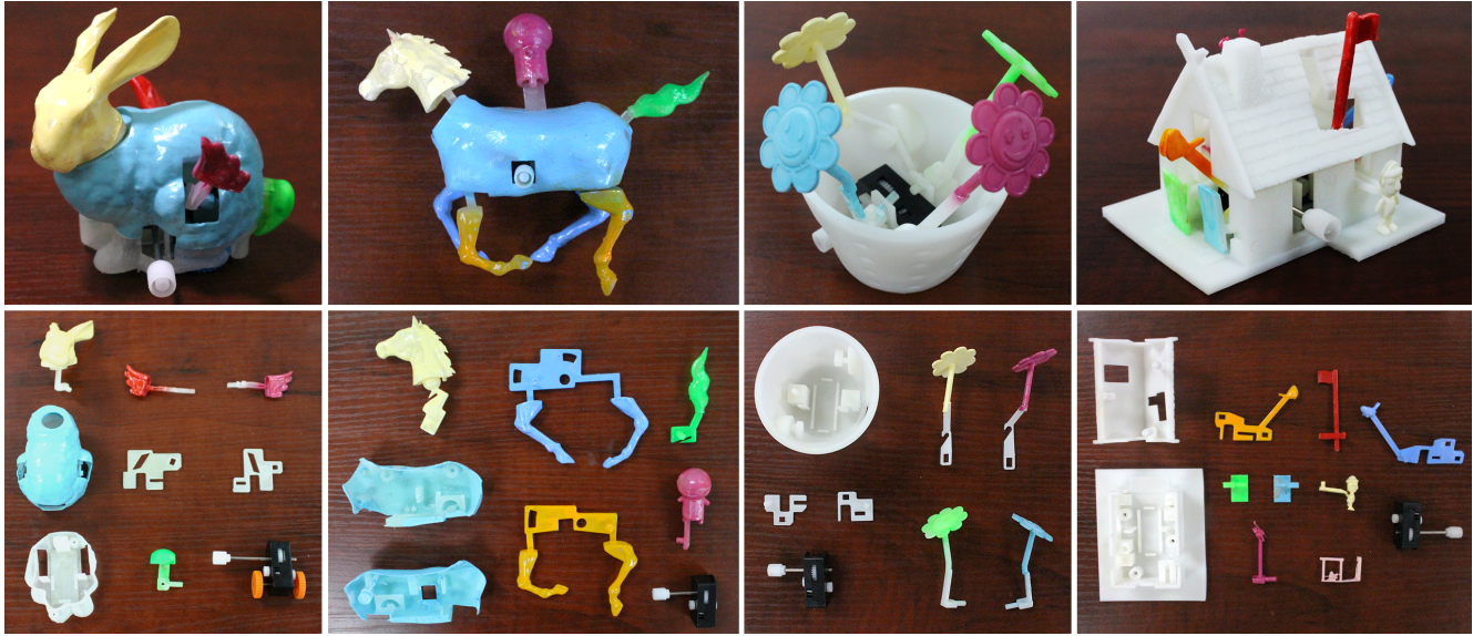
Fig. 18. Four of the six wind-up toys (top) that we have fabricated and assembled from 3D-printed parts (bottom). From left to right: BUNNY (13.0g shell + 7.8g motor + 9.0g mechanism), HORSE (15.3g shell + 5.9g motor + 26.1g mechanism), FLOWER POT (34.8g shell + 5.8g motor + 8.0g mechanism), and HOUSE (48.9g shell + 6.0g motor + 6.4g mechanism). See their statistics in Table 3.
