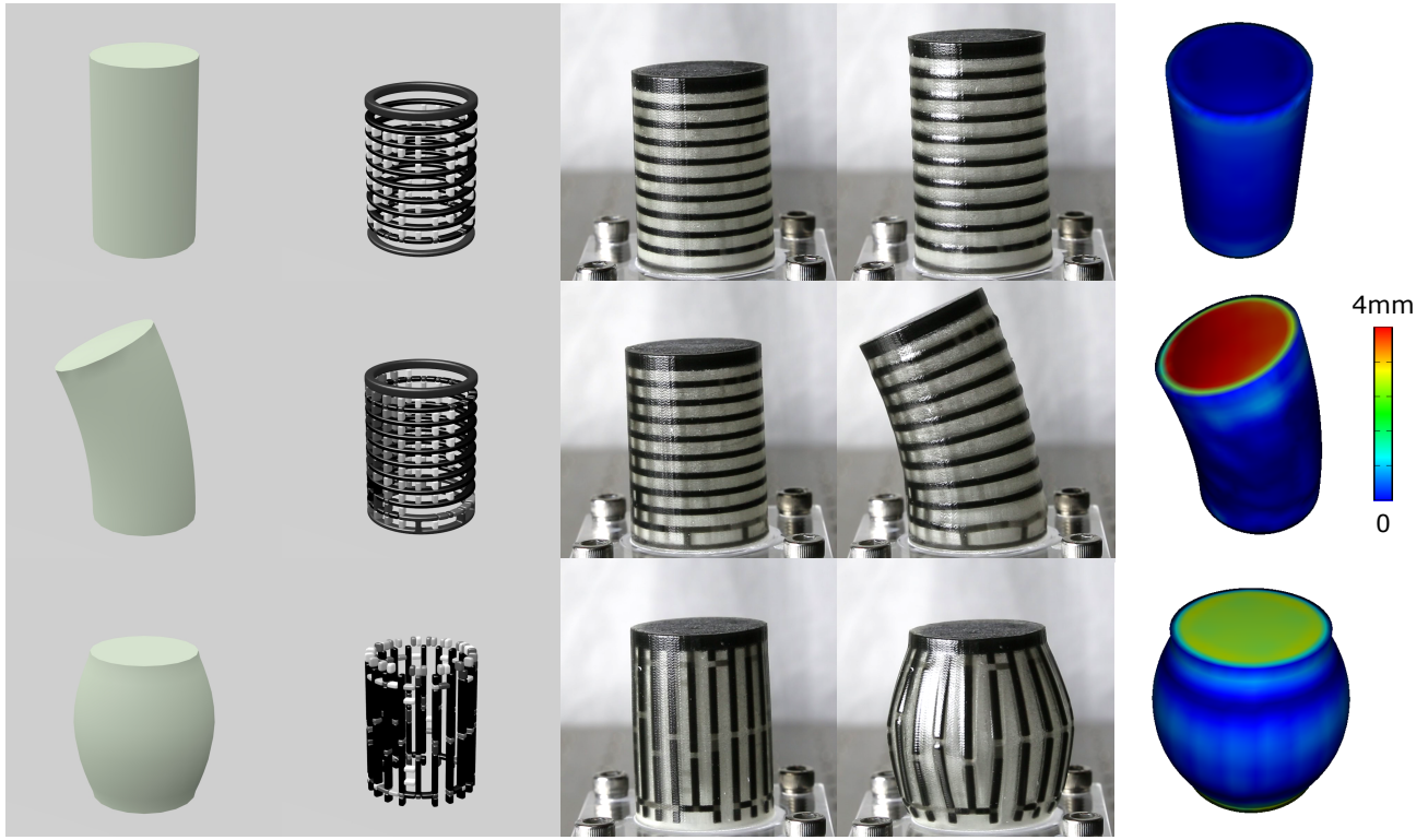
Fig. 5. Cylinder model. From left to right: target shape, the frame structure whose color encodes the material type (for frame segments with the base soft material, they are not rendered), the fabricated object at the rest pose, the inflated object, the color coding of geometric errors between the inflated object and the input target shape.
