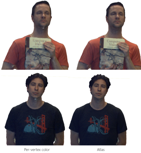
Fig. 10. Per-vertex Color Compared to Atlas Mapping. With the voxel resolution fixed, per-vertex colors look blurred and suffer from block artifacts. Increasing the voxel resolution to alleviate this issue is computationally inefficient. On the other hand, atlas mapping decouples geometry resolution from color quality.
