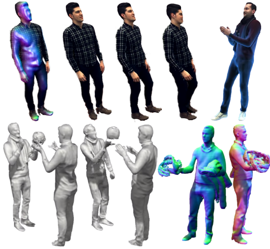
Fig. 2. Screenshots from Holoportation [Orts-Escolano et al. 2016] and Fusion4D [Dou et al. 2016] videos. Geometric over-smoothing leads to uncanny reconstructions especially of faces (top row). Fast motions are supported but by degrading to noisy data samples in that region c.f. the scarf of the user (bottom right). Topological changes are also handled by localized resetting of the data c.f. the ball (bottom left).
