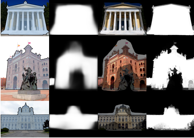
Figure 6: Qualitative analysis of matting improvements to segmentation. From left to right, we show the input image with the manually labeled ground truth, the MaskRCNN output, the generated trimap, and the output of alpha matting. Best viewed with zoom.
